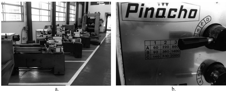
FIGURE 1. PINACHO LATHE a. U PASCUAL BRAVO MACHINE AND TOOLS LABORATORY. b. RPM SELECTION MODE.
